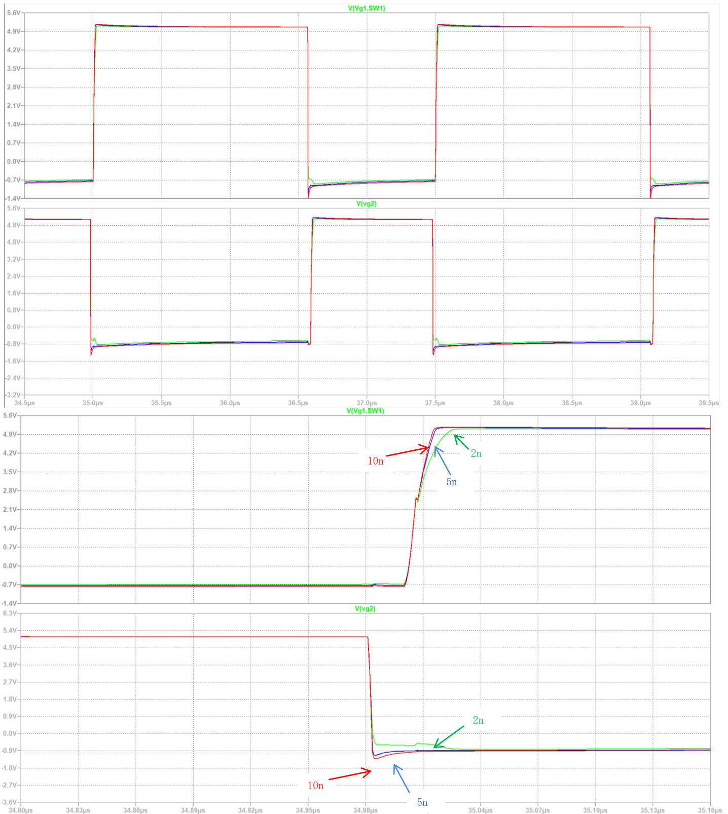
Figure 10 Effect of different capacitance values on driving waveforms
